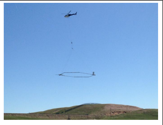
Photo of the helicopter-assisted SkyTEM304 performing the AEM survey above the Belvoir Ranch. May 31, 2017.
